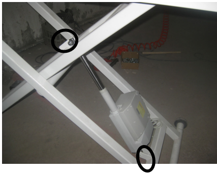
The clamp-spring at both-end of the actuator
