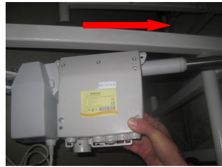
<1> Slide the control box upward to split it from the actuator
