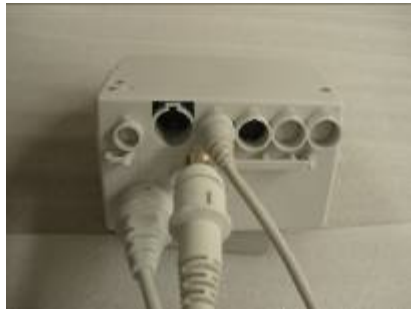
The foot-control-plug is at the end of the cable. The socket is on the control-box.
