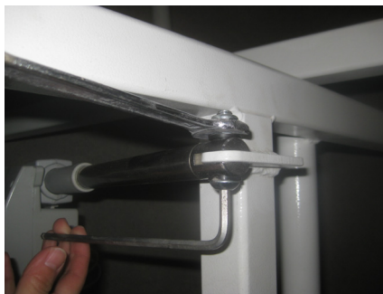
<2> Remove the clamp spring and the bolt
